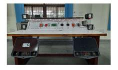
This lab also consists of different types of Single/Multi/Dual (High Availability) digital axle counters of CEL, GGtronics, Medha, Eldyne makes. The trainee will be able to study the general architecture of the system, their functions and system power supply requirements. The trainees will be able to appreciate the advantages of Digital axle counters over conventional track circuits. Trainees will be able to know the
